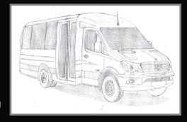
THE SPRINTER BUS FEATURES A GALVANEEL STEEL FRAME BODY FOR MAXIMUM BODY STRUCTURAL DURABILITY AND PRODUCT LONGEVITY. THE REAR LUGGAGE AREA'S FLOOR DROPS BELOW THE BUS FLOOR TO ALLOW FOR MAXIMUM LUGGAGE CAPACITY WHILE PROVIDING LARGER AISLE SPACES AND A ROOMY ATMOSPHERE FOR PASSENGERS.
