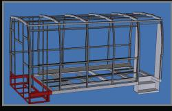
Rear Luggage compartment floor goes beneath Sprinter Bus floor to maximize passenger space without taking away luggage space.
