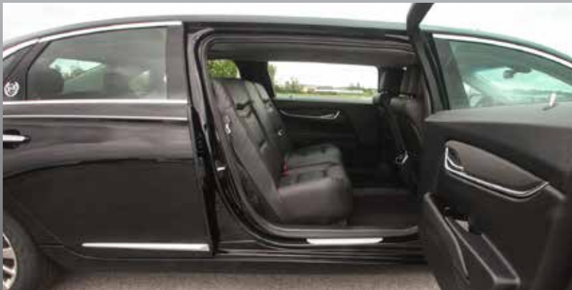
The center door's 88 degree hinging greatly eases entry and exit while its interior panel is trimmed in full Cadillac style.
